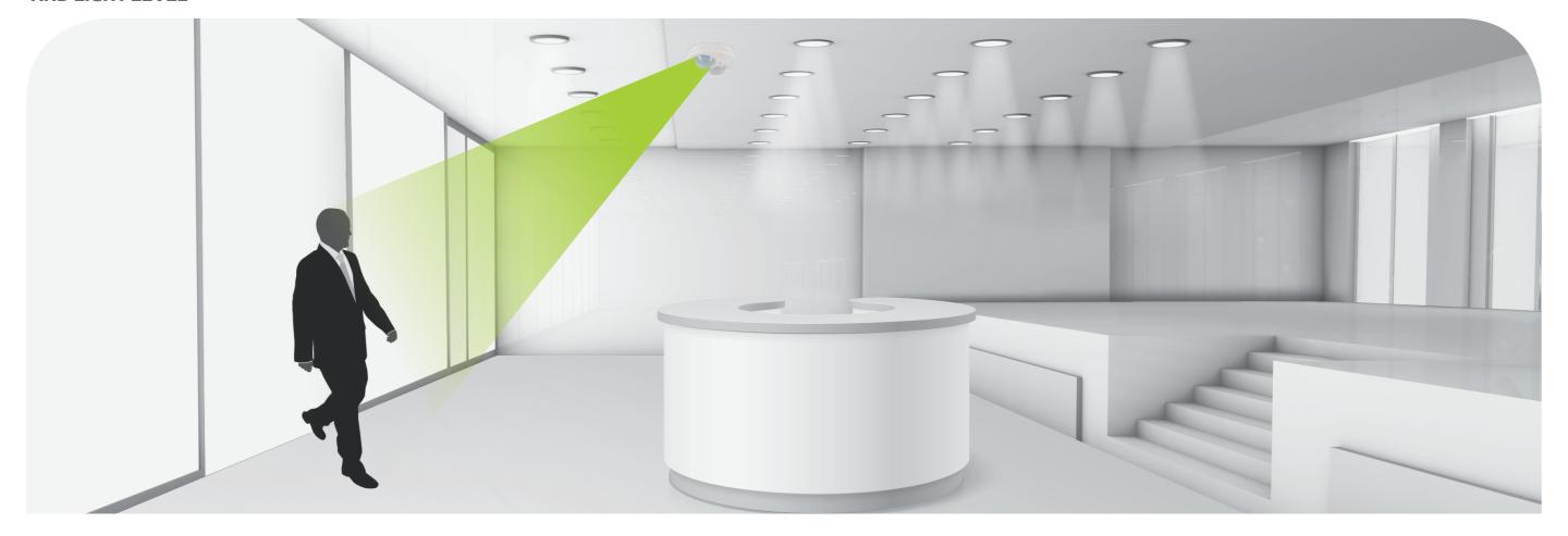
You can set your lighting automatically according to motion and the level of light in the room. For example on sunny days the light can be turned down and then turned up again to full capacity on cloudy days. In areas where no motion is detected the lights will not stay on unnecessarily providing energy efficiency.
